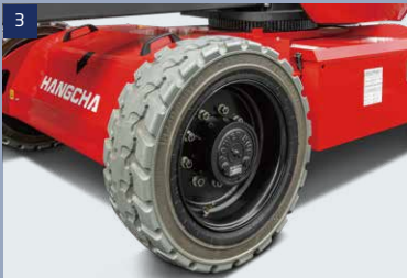
Tires: foam-filled tires with good off-road performance
